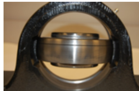
Figure 4 — Torquing bearing 90° into housing
