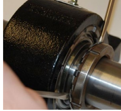
Figure 2 — Zero Shaft Fit: Pry against housing to draw adapter sleeve through bearing. Sleeve should not be protruding out the backside of the inner ring.
