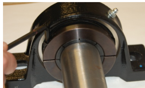
Figure 1 — Set screw tightening on a Centrik-Lok bearing
