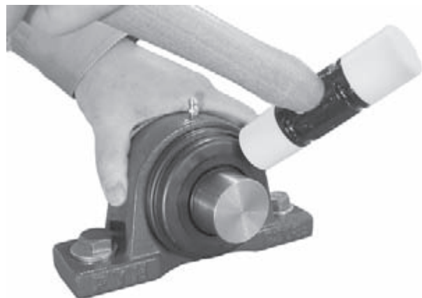
Fig. 14.13 Installing steel plate covers
