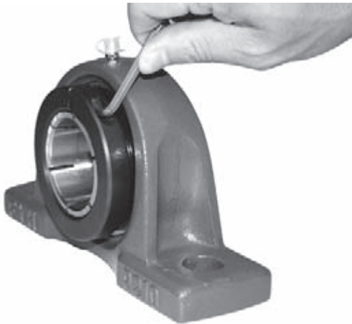
Fig 14.11 Installation of NU-LOC units
